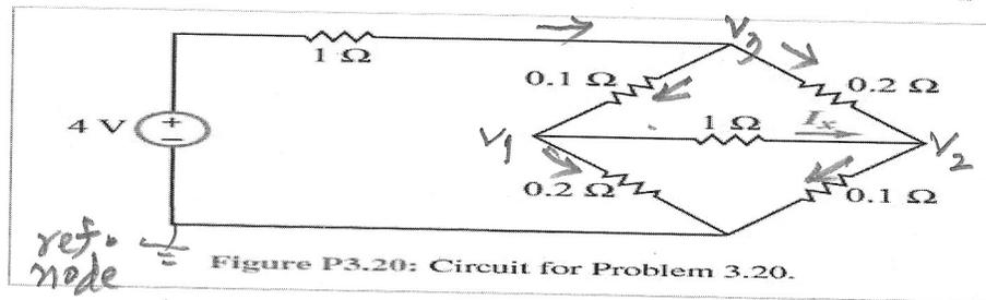
Part A (4 points) Let us solve for  $I_x$  as  $I_x = \frac{V_1 - V_2}{1\Omega}$ , where the two voltages are node voltages at both ends of the  $1\Omega$  resistor through which  $I_x$  flows. Write down two KCL equations to solve for  $V_1, V_2$ .
