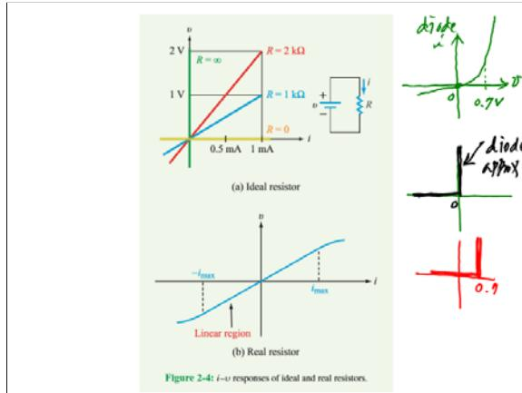
Figure 2-4:  $i$ - $v$  responses of ideal and real resistors.
