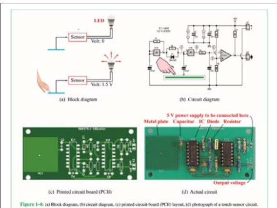
Figure 1-4: (a) Block diagram, (b) circuit diagram, (c) printed-circuit-board (PCB) layout, (d) photograph of a touch-sensor circuit.
