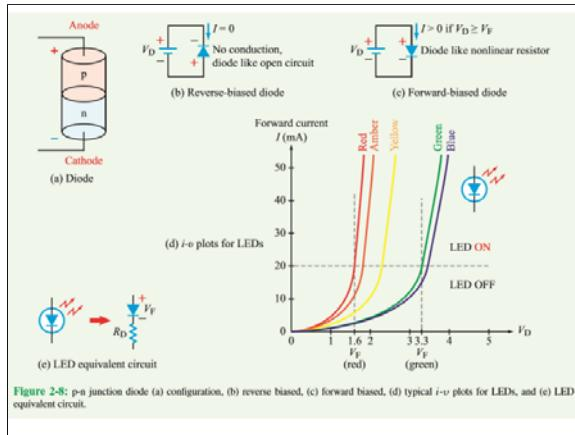
Figure 2-8: p-n junction diode (a) configuration, (b) reverse biased, (c) forward biased, (d) typical  $i$ - $v$  plots for LEDs, and (e) LED equivalent circuit.
