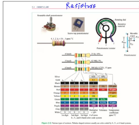
Figure 2-2: Various types of resistors. Tubular-shaped resistors usually are color-coded by 4-, 5-, or 6-band systems.
