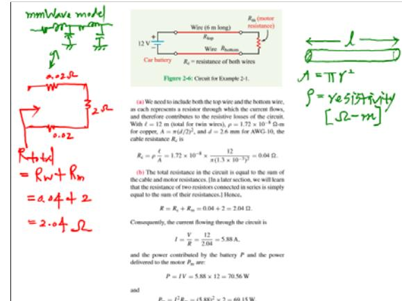
Figure 2-6: Circuit for Example 2-1.
