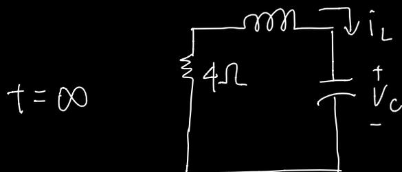
At the beginning of the stage, the circuit is at steady state, and the inductor behaves like a short circuit, the capacitor behaves like an open circuit. As a result,
