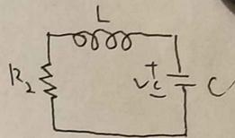
$$\text{When } t > 0 \quad \begin{cases} R_2 I_C + L \frac{dI_C}{dt} + V_C = 0 \\ I_C = C \frac{dV_C}{dt} \end{cases} \Rightarrow R_2 C \frac{dV_C}{dt} + LC \frac{d^2 V_C}{dt^2} + V_C = 0 \quad (1)$$
