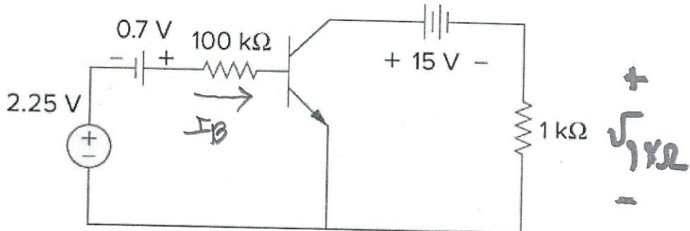
Answer  $V_{1\text{k}\Omega} = -2.25 \text{ [V]}$  Power =  $5.06 \text{ [mW]}$
