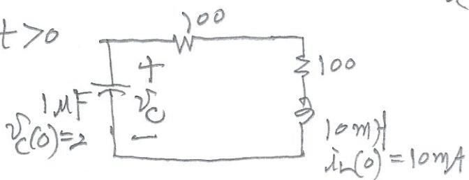
$$v_C = i_L(100+100) + 10 \times 10^3 \frac{d}{dt} i_L \quad (1) \quad \text{where } i_L = -\dot{v}_C$$
