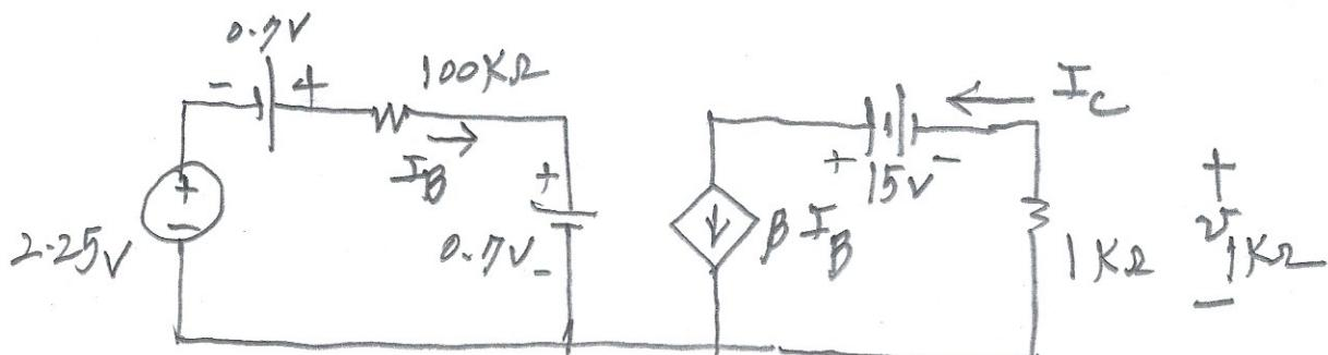
Using Mesh analysis;  $-2.25 - 0.7 + 100\text{k}\Omega I_B + 0.7 = 0$
