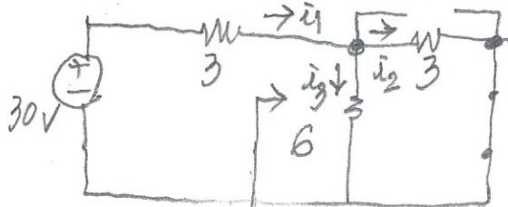
$$\begin{cases} i_1(0-) = \frac{30 \text{ [V]}}{(3+2) \text{ [Ω]}} = 6 \text{ [A]} \\ i_2(0) = i_L(0) = 6 \times \frac{6}{6+3} = 4 \text{ [A]} = i_L(0) \\ v_C(0) = 3 \times 4 = 12 \text{ [V]} = v_C(0) \end{cases}$$
